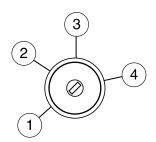
3. Turn the ignition to the 1 (off) position and remove the first **coded key** from the ignition.
